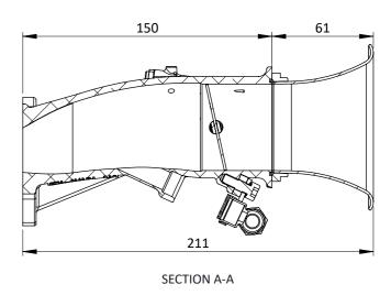
This is the Jenvey BMW E30 M3 direct to head kit (DTH). The kit has Ø52mm brass throttle bodies, underslung fuel rail, linkage bracket and AHD 52X60 air horns.
